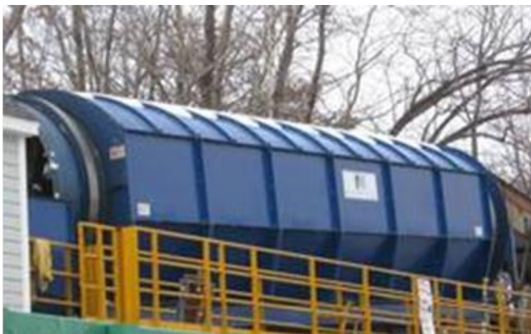
Figure 2-9 Trommel Screen Processing MSW
